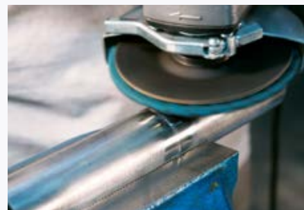
Sanding fine welding seams and removing thermal discolouration
